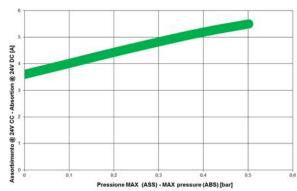
NOTE: Graph shows inlet pressure at a temperature of 20°C (tolerance ±10%)
